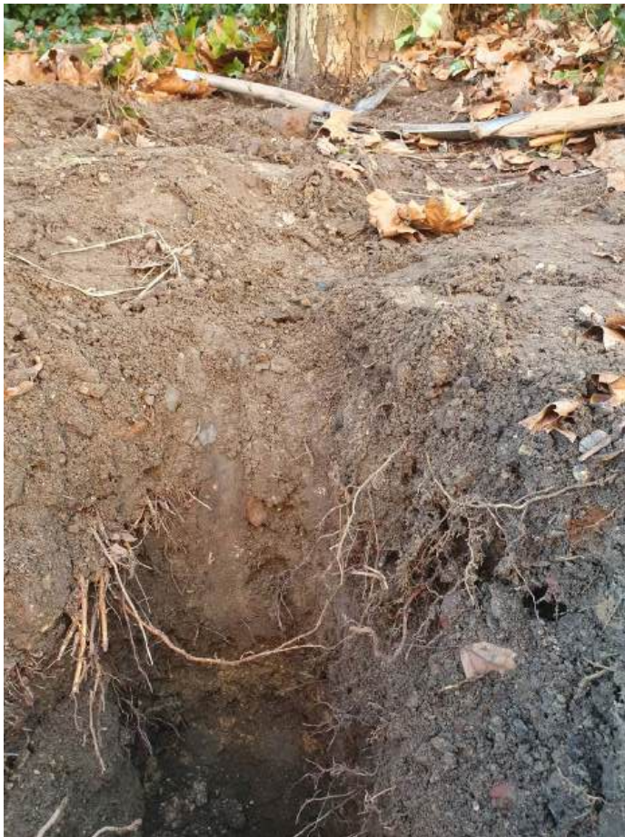
Figure 3 (K. Dupon). Manually digging the soil to assess the root system and the soil.
