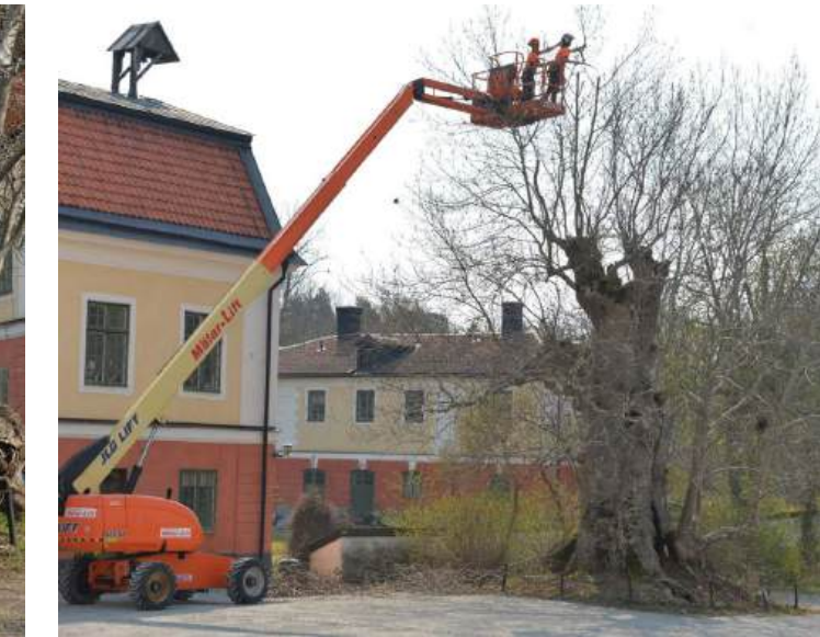
Figure 5 (D. Daggfeldt). An articulated boom lift with a 25-metre reach was used to access the top of the crown without unnecessarily compacting the ground within the root protection area. The pruning was carried out by handsaws using the "cut-and-hold" technique to prevent damage to the tree caused by falling branches.
